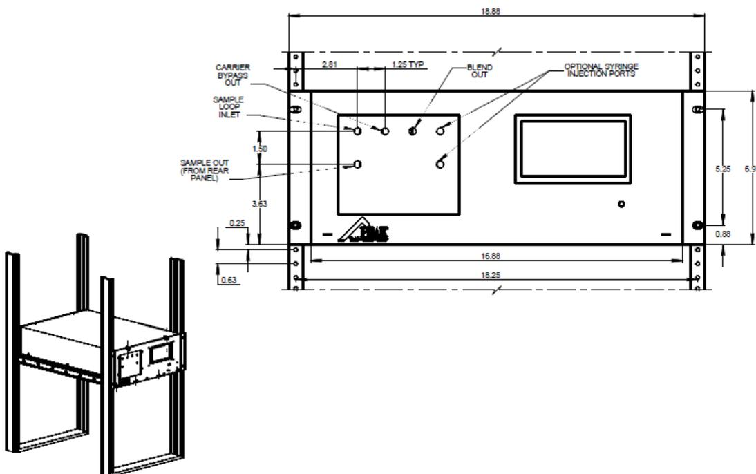
Figure 2. Rack Mount Front View with Dimensions
