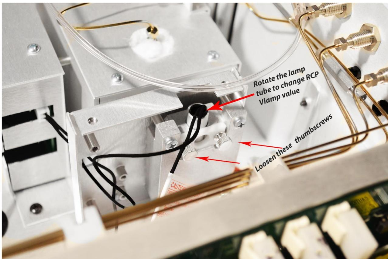
Figure 78. UV Lamp Adjustment
