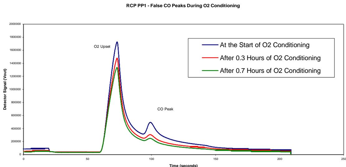
Figure 68: False CO Peaks Created by Free Carbon on the Column Materials
