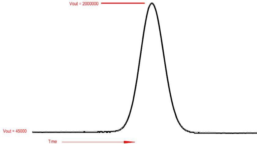
Figure 57. Typical Chromatographic Detector Signal Showing a Peak
