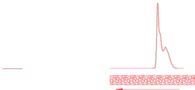
Figure 44. Peak Development on the Analytical Column Soon After Injection
