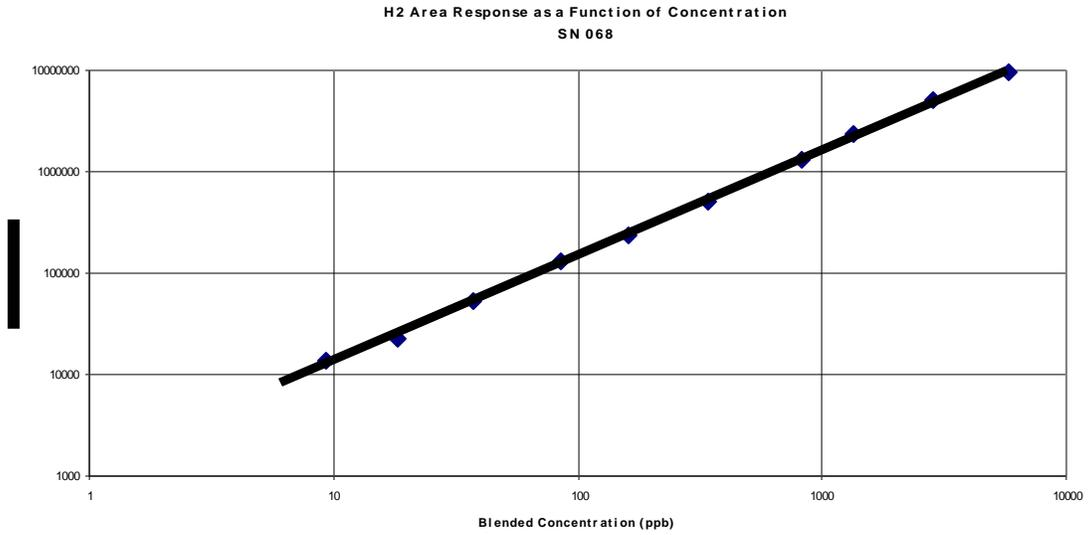
Figure 73. Typical Area Response Curve for Hydrogen, Showing Linear Range
