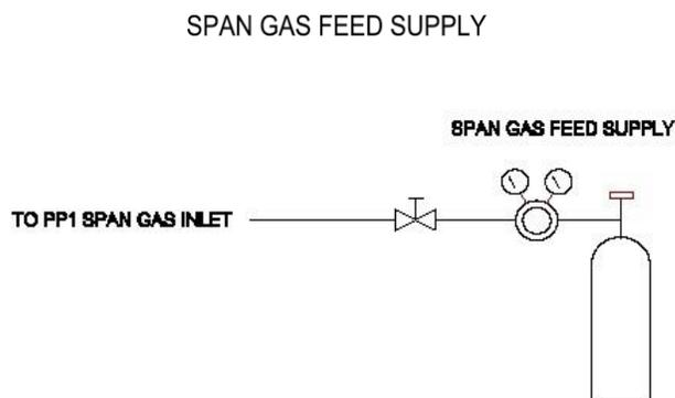
Figure 8. Span Gas Supply Flow Schematic
