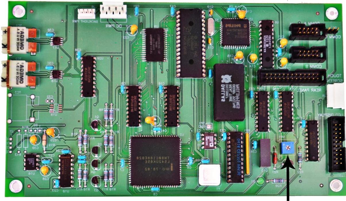
*Adjust this potentiometer to change display intensity and contrast*
