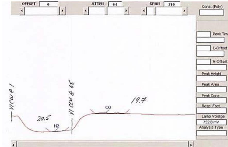
Figure 51. High FID flow from NV1 (note rise after the V1 CCW command)
