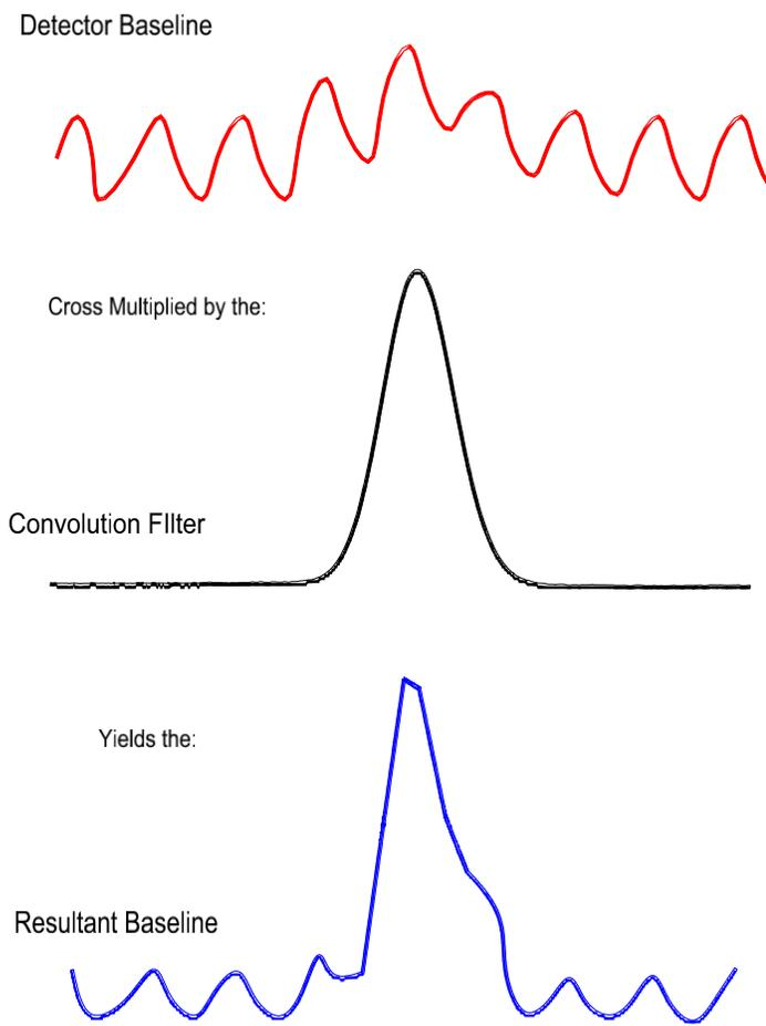
Figure 61. Convolution to Enhance Signal Characteristics
