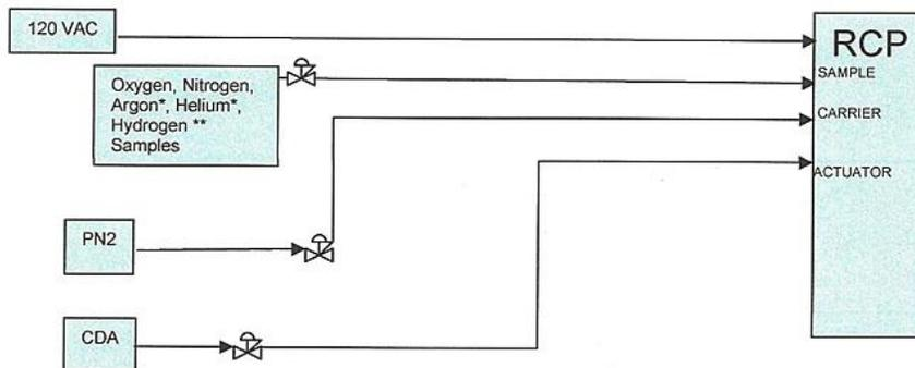
Figure 6. RCP PP1 Gas Supply Schematic
