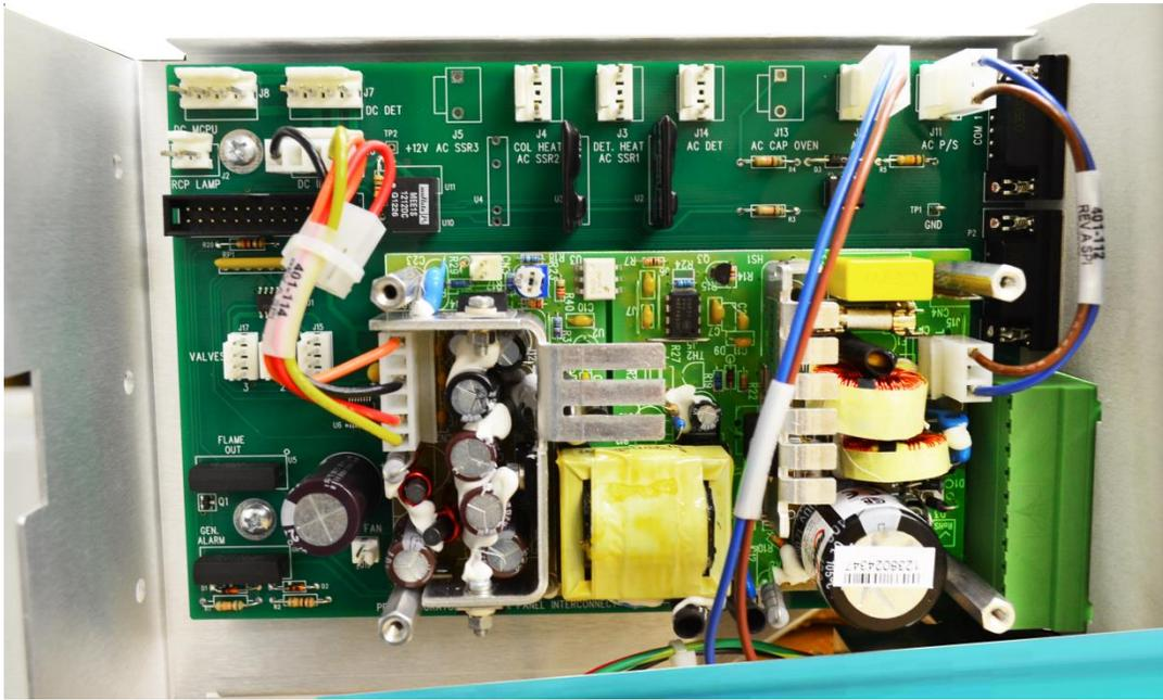
Figure 83. Main DC Power Supply with Shield Removed
