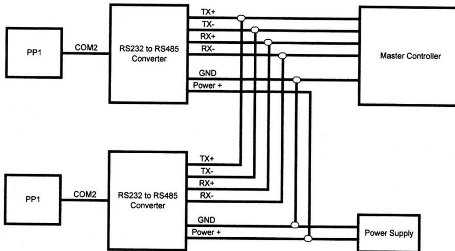
Figure 42. System configuration diagram with basic connections.
