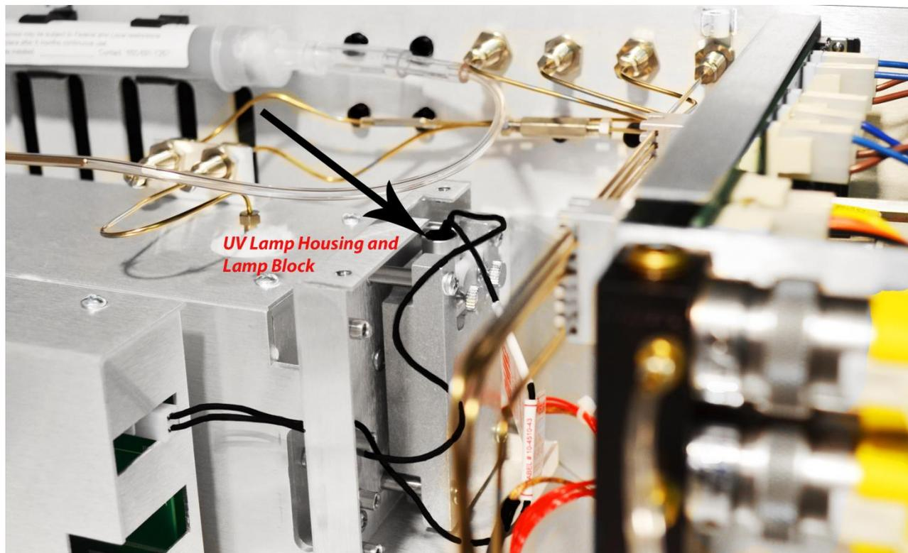
Figure 77. Location of the UV Lamp (Protective cover removed)
