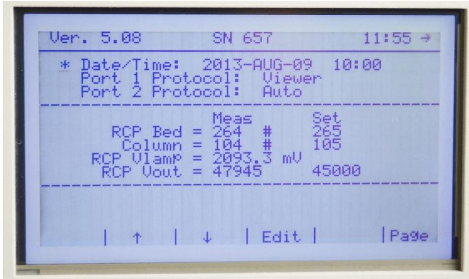
Figure 11. Set-up (or Main) Screen – Upper Section
