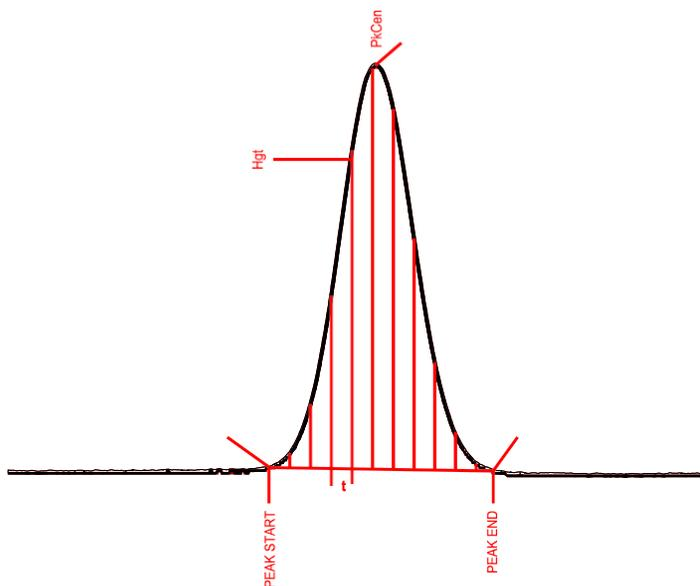
Figure 58. Illustration of Measurement of Chromatographic Peak Area
