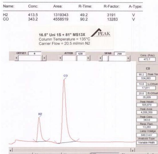
Figure 55. Effect of 30C Increase in Column Temperature
