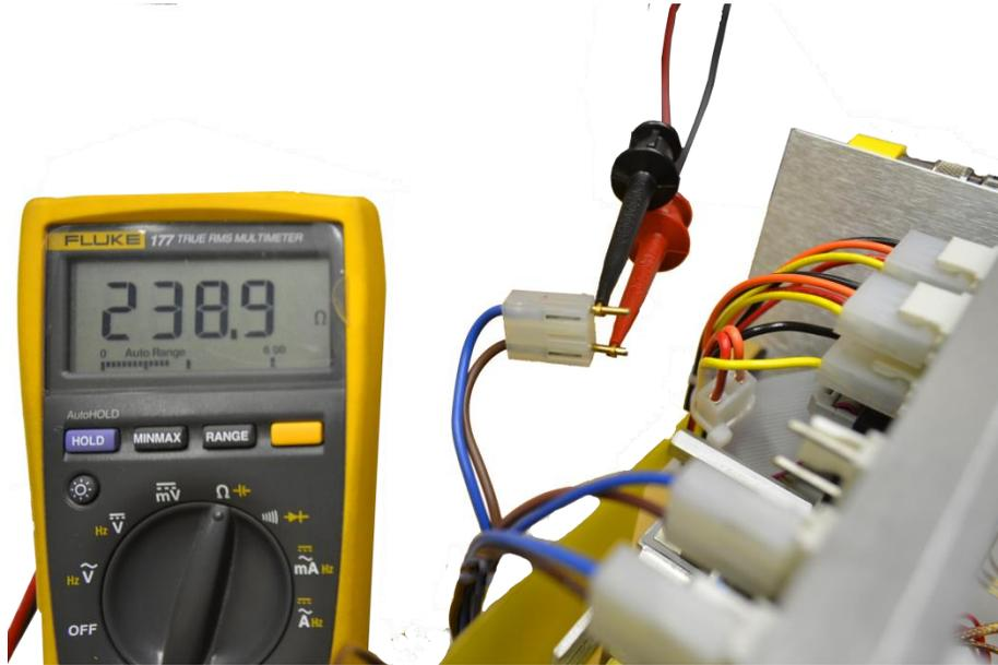
Figure 80. Heater Resistance for 90 – 120 VAC AC Service
