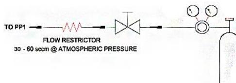
Figure 7. Sample Supply Flow Schematic
