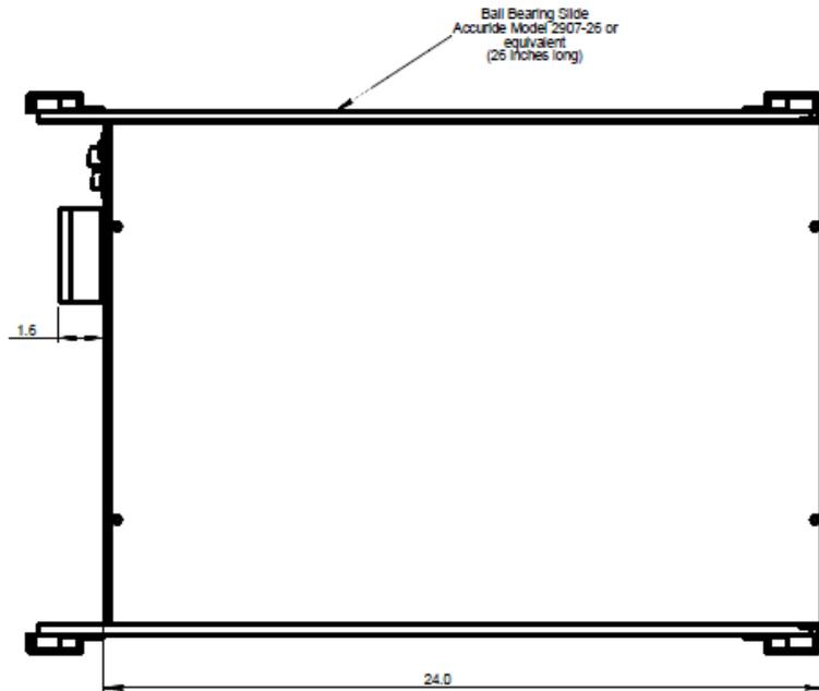
Figure 4. Rack Mount Top View with Dimensions
