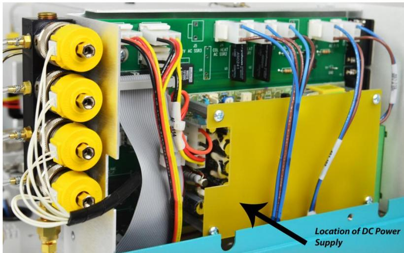
Figure 82a – Main DC Power Supply Location
