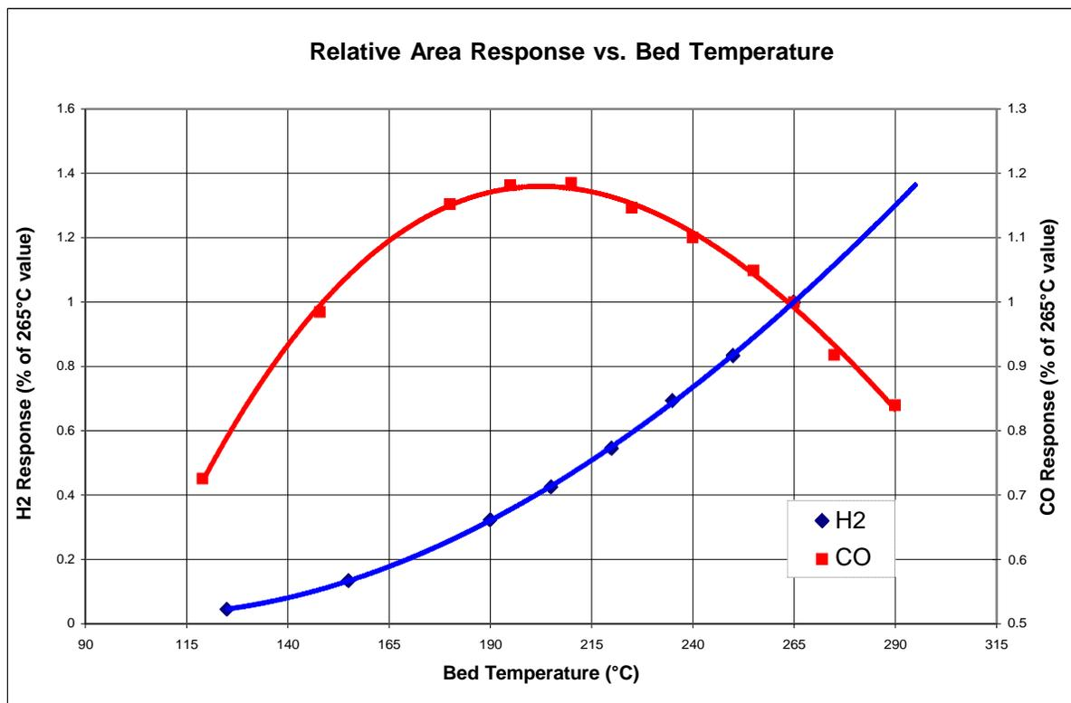
Figure 71. RCP Temperature Response for H2 and CO
