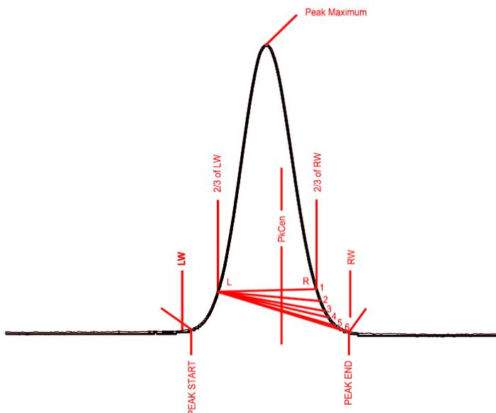
Figure 66. Progression of Peak End Time Calculation
