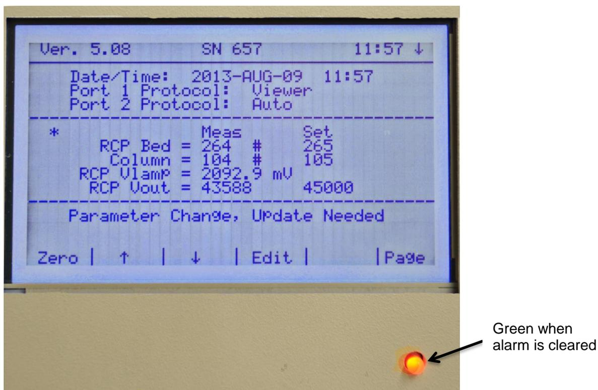
Figure 14. Set-up Screen Displaying an Error Message
