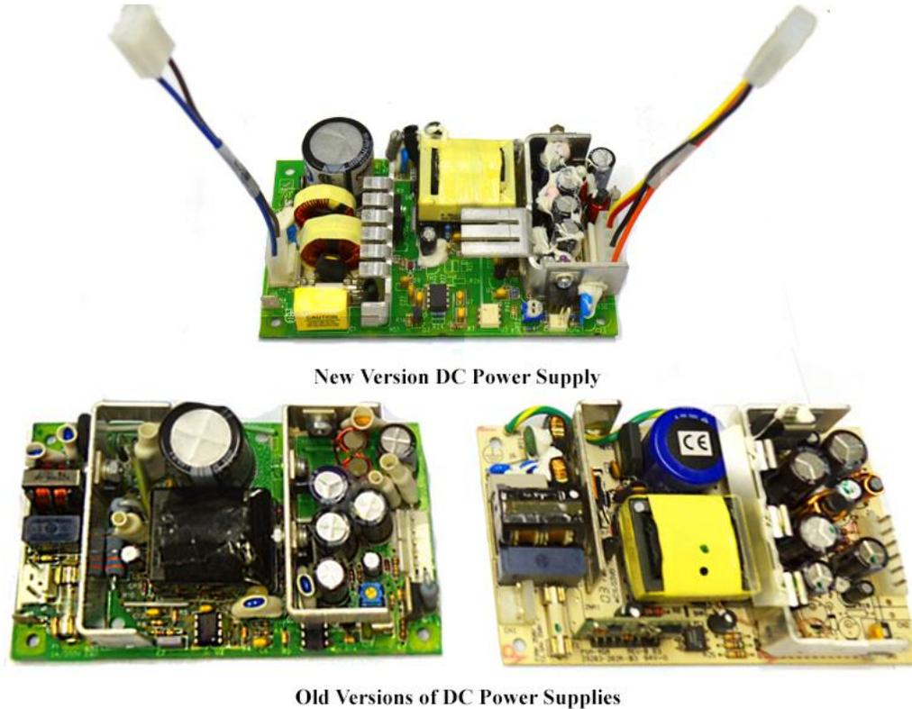
Figure 85. Correct Alignment and Cable Transfer from Old to New DC Power Supply
