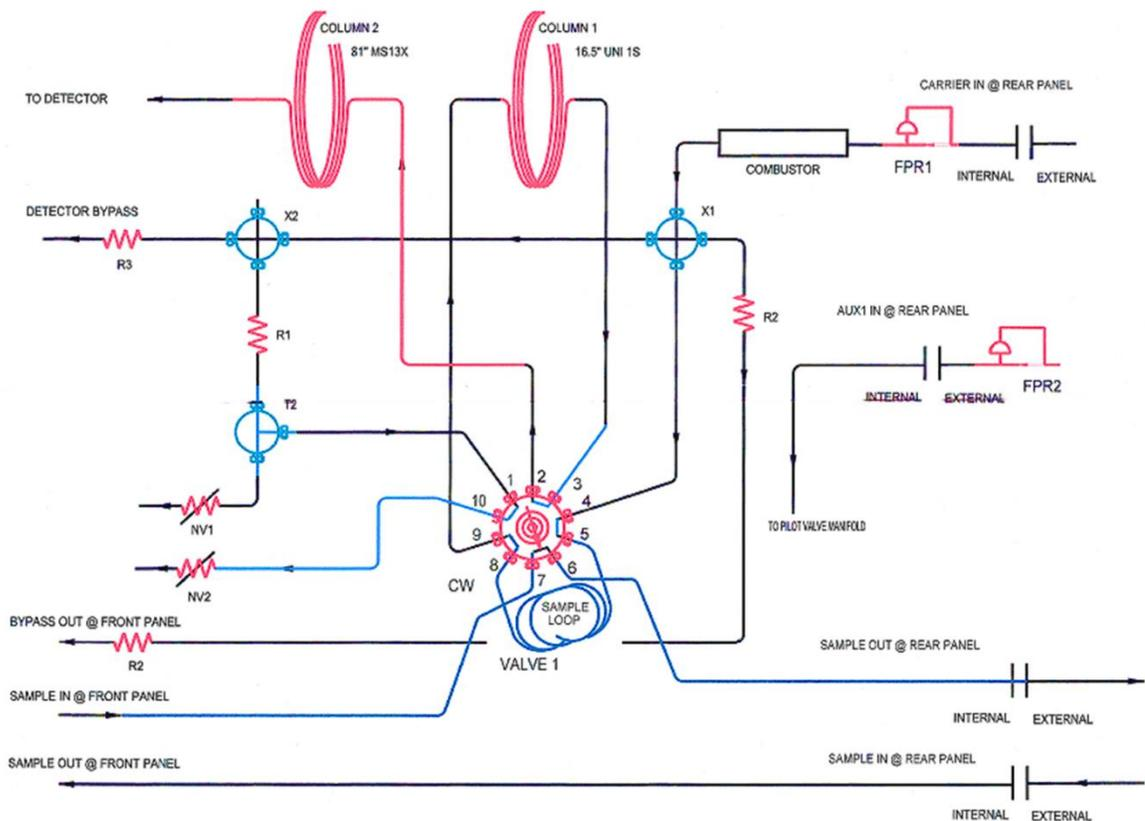
Figure 43. Typical RCP plumbing diagram
