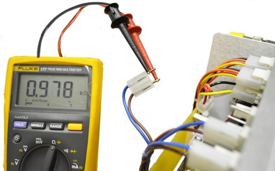
Figure 81. Heater Resistance for 200-240 VAC AC Service
