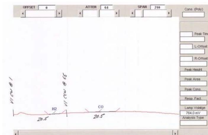
Figure 50. Properly Flow Balanced Baseline
