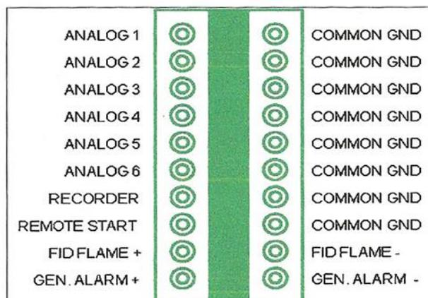
Figure 19. Analog Output Connections
