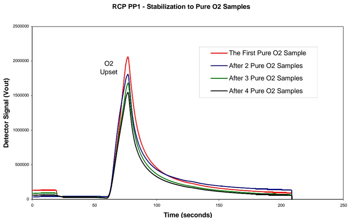
Figure 69. A Sequence of Pure O<sub>2</sub> Sample Chromatograms Showing Improvements With Additional Injections
