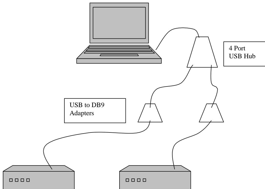
Figure 88. Multiple Analyzers Connected to a Single Computer For Using Viewer Software
