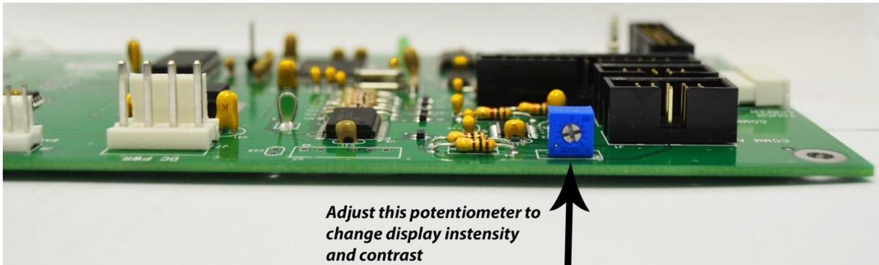
*Adjust this potentiometer to change display intensity and contrast*
