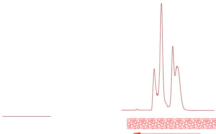
Figure 45. Peak Development Midway on the Analytical Column
