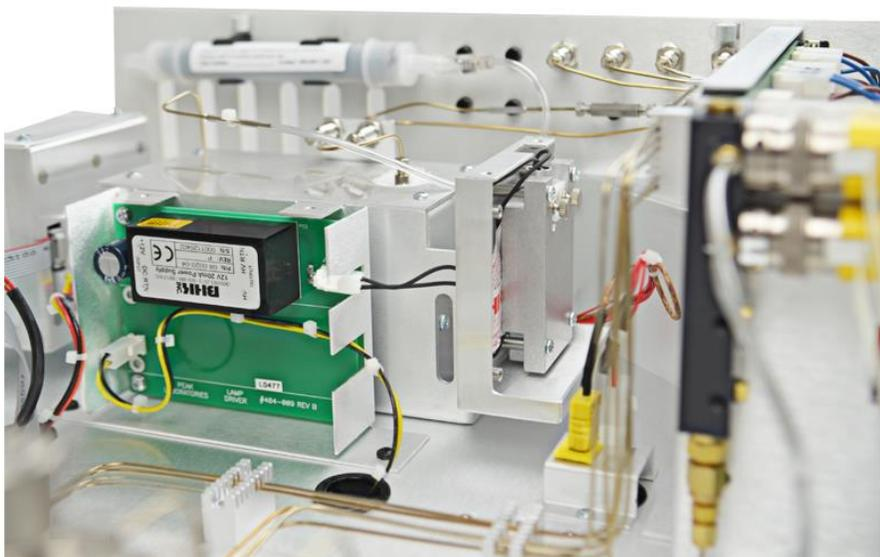
Figure 9. RCP Detector Showing Column Outlet and Standby Fittings
