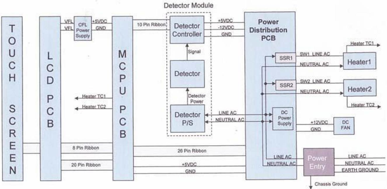
Figure 76. PP1 Functional Block and Interconnect Diagram
