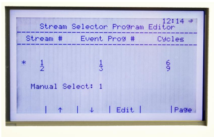
Figure 25. Stream Selector Sequence Screen
