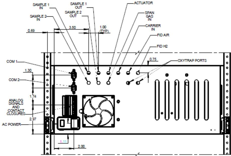
Figure 3. Rack Mount Rear View with Dimensions
