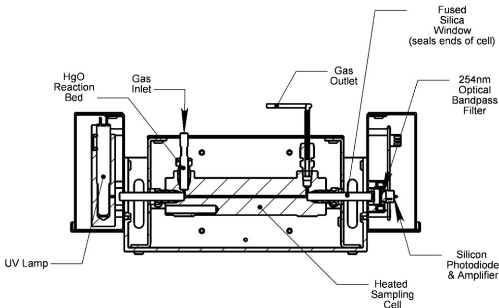
Figure 70. Standard RCP Section
