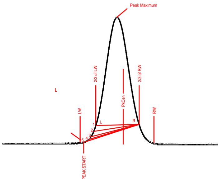
Figure 65. Progression of Peak Start Time Calculation
