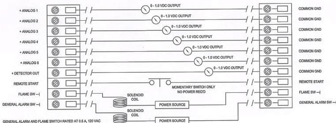
Figure 20. Analog Output Wiring Schematic
